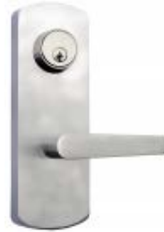
VSEA 410 Escutcheon Lever Trim Non handed Free wheeling, clutch design Stainless Steel 304 Door Thickness: 45-50mm Finish: SS, PSS, PVD, AB
